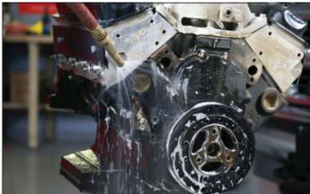
VpCI®-414 effectively removes dirt, oils, and greases or other cosmoline-like products.
